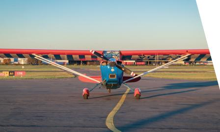
Lycoming AEIO-360-H1B Analogue Avionics with Dials + EFIS D10A Aerobatic Category MTOW: 886kgs Cruising Speed 120kts Aerobatic Rating +6/-5G 2 Seater (Tandem)
