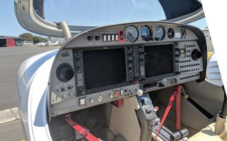
Continental CD-135 Engine x 2 FADEC single lever power controls Garmin G1000 Avionics Maximum Take-Off Weight (MTOW) 2000kgs Cruising Speed 150kts @ 60% Power 4 Seater
